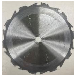
Cutting blade with diamond chip
